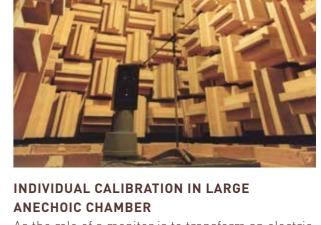
As the role of a monitor is to transform an electric signal into an acoustic signal, every single monitor produced is checked and calibrated in our large anechoic chamber to ensure its quality.
