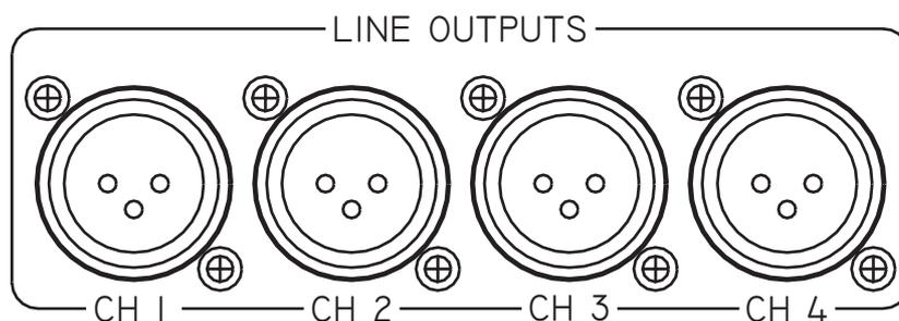
Any professional level balanced audio input sources can be connected to the analog line outputs of the DUA II. 4 output levels are selectable from consumer level (–10 dBV) up to professional level (+4 dBu).
