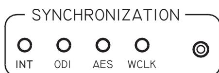
The DUA II can operate in many different synchronization modes. It can synchronize to its internal clock or to a wide range of industry standard external sources. Pressing the *SYNCHRONIZATION* button allows the selection of the desired synchronization mode.
