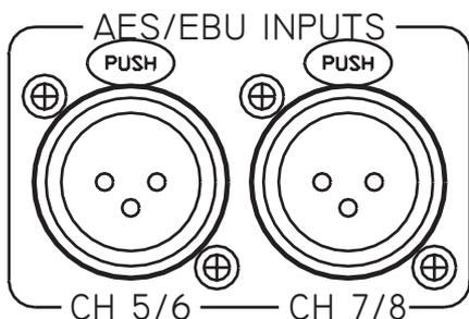
Any professional level balanced digital AES/EBU audio output sources at 32, 44.1 or 48 KHz can be connected to the AES/EBU inputs of the DUA II.
