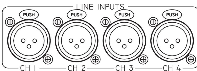
Any professional level balanced audio outputs sources can be connected to the analog line inputs of the DUA II. 4 input levels are selectable from consumer level (–10 dBV) up to professional level (+4 dBu).
