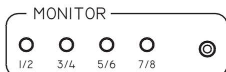
This section allows for the Selection of any of the 8 input or output audio signals in pairs. The desired monitoring source is selected by pressing the *MONITOR* button.
