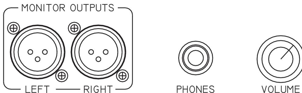
Any professional level balanced audio input can be connected to the analog line monitor outputs of the DUA II. 4 output levels are selectable from consumer level (-10 dBV) up to professional level (+4 dBu). See chapter 4 on how to configure the *Analog Outputs Level*.
