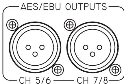
Any professional level balanced digital AES/EBU audio inputs at 32, 44.1 or 48 KHz can be connected to the AES/EBU outputs of the DUA II.
