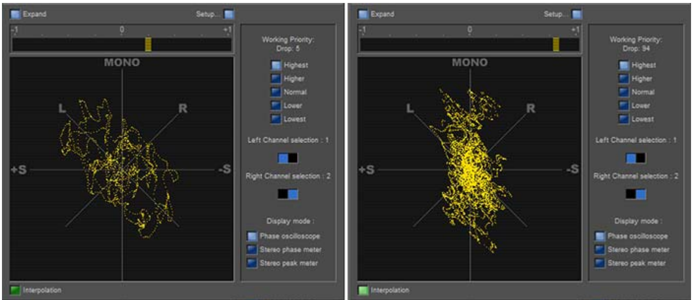
Phase oscilloscope without and with Interpolation
