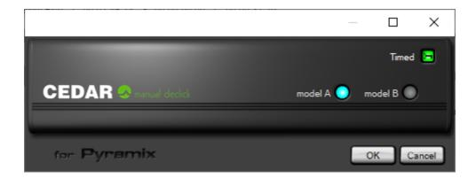
Manual declick should be used to remove extended clicks. It allows you to specify the audio that constitutes the click and restores the audio using an interpolator that is optimised for longer clicks and scratches. The maximum click length handled is approximately 0.1s irrespective of sample rate.
