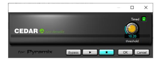
Auto decrackle removes surface noise, crackles, and some types of buzz. You may also use it to reduce the audible effects of amplitude distortions caused by problems such as microphone diaphragm grounding and over-driven mixer inputs. It is an almost foolproof process. However, it will only function correctly if there are no major ticks or clicks received at the input. If obvious clicks exist within your material they must be removed before processing the audio using Auto decrackle.
