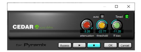
Auto Dehiss embodies an advanced algorithm that offers a unique Auto mode that enables the software to determine the noise content of the recording and remove this with minimal loss of high frequencies and without the introduction of unwanted artefacts. It offers two modes:
