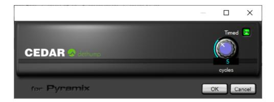
Dethump should be used to remove low frequency disturbances. The maximum thump length handled is approximately 1s irrespective of sample rate.
