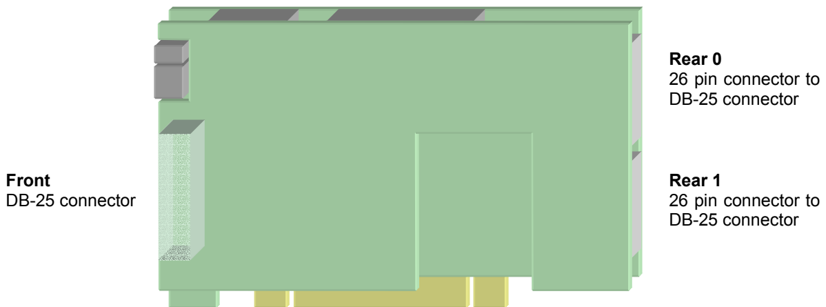
Figure 12 - Location of the on-board connectors on the AES, SDIF & TDIF daughter cards
