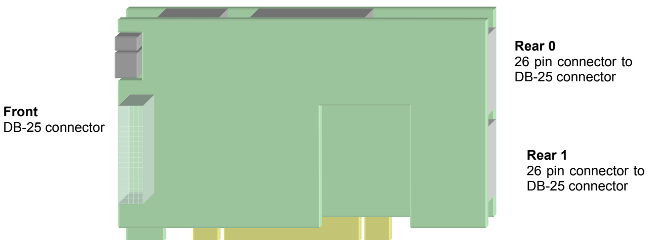
Figure 16 - Location of the on-board connectors on the AES, AES II, SDIF & TDIF daughter cards
