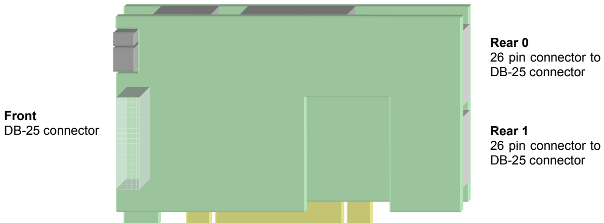
Figure 11 - Location of the on-board connectors on the AES, SDIF & TDIF daughter cards
