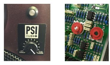
When assembling the back panel to the cabinet, take great care in positioning the level axis into the potentiometer. This can be quite tricky and the best is to use a light to see the axis through the level hole on the back panel.
