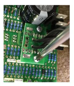
On the A14, the level axis needs to be attached to the potentiometer Make sure the Level axis in turned to "cal" Make sure the potentiometer is also in "cal" position
