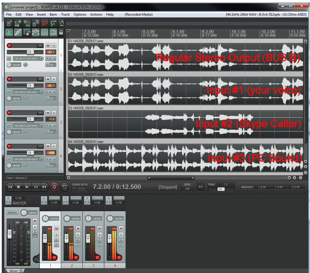
REAPER recording 4 stereo tracks coming from Voicemeeter virtual ASIO output.
