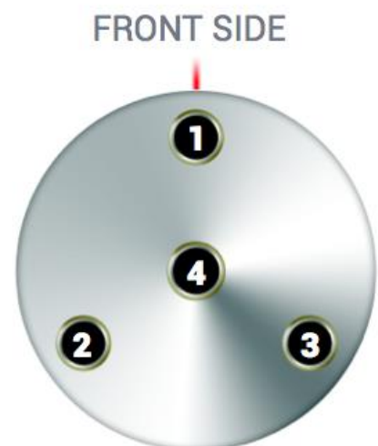
The calibration microphone and the arrangement of the capsules
